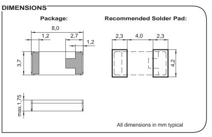
Suitable for Downhole application SMT ceramic package height 1.75 mm Fundamental mode up to 24MHz Extremes temperature ranges High stability and low aging High shock and vibration resistance Hermetically sealed Ultra low MSL Excellent solderability Swiss made quality Customer specification on request
